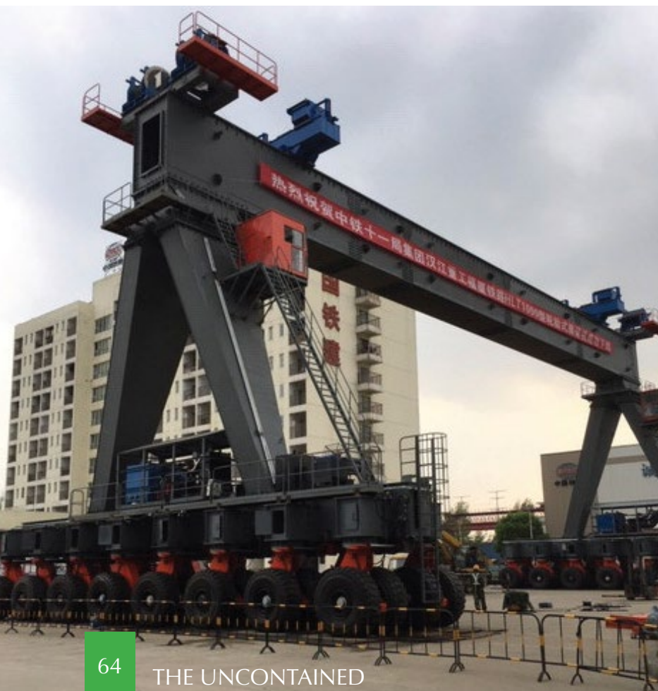
[image 3.11-1] 450 ton beam lifting machine manufactured by HHI ready for shipment to Putian city, Fujian for HSR construction
